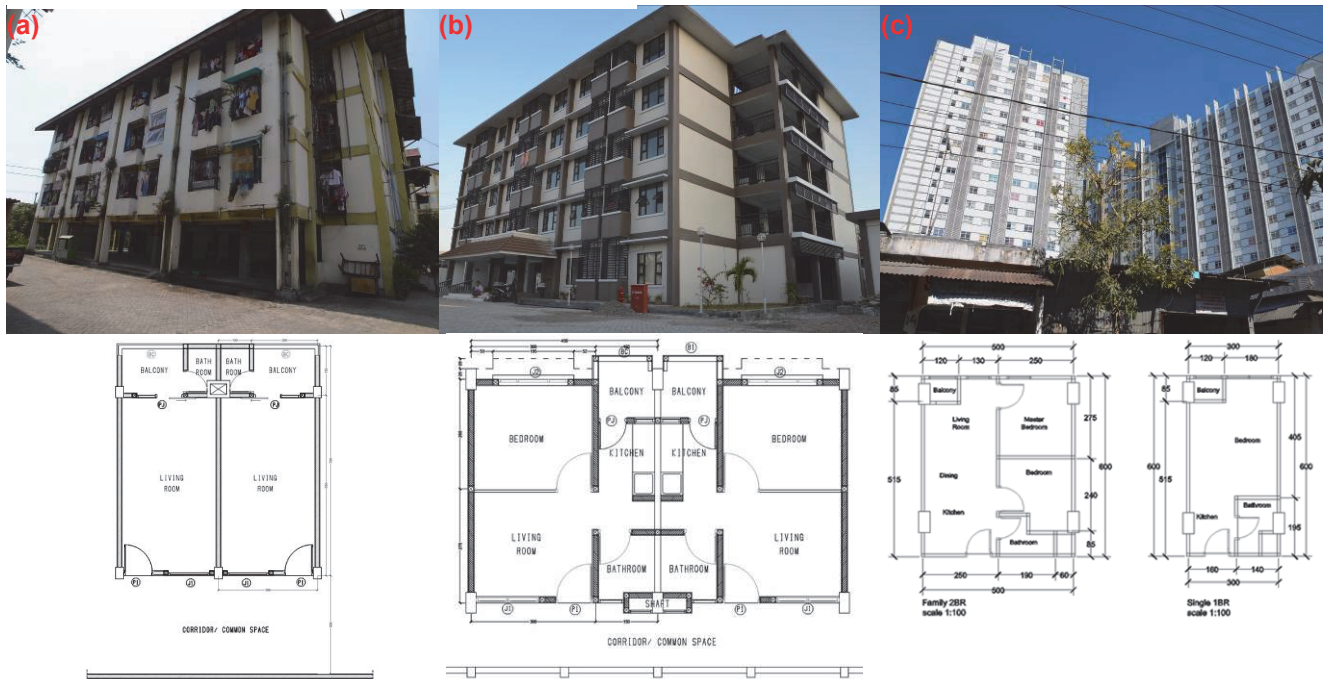
Fig. 2 Sample of apartments from each category and the typical unit plan: (a) Old public apartment; (b) New public apartment; and (c) Private apartment
